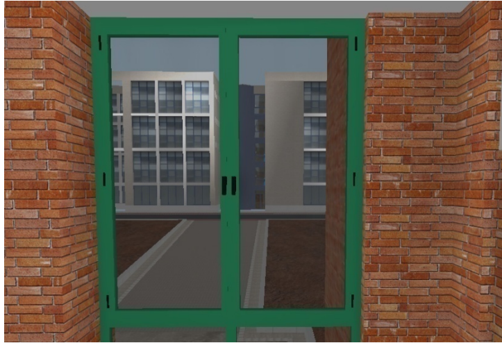
Fig. 25. Window with only frame, hinges, handle and glass
