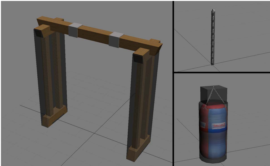
Fig 46. Punching bag elements with their collision hulls
