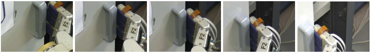
Fig. 14 A sequence showing the vision-tactile-force alignment process during task execution, starting from a coarse initial position.
