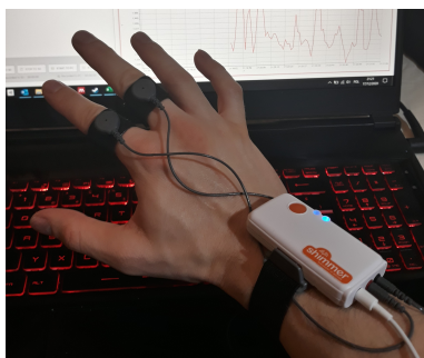
Figure 17: Shimmer GSR device attached on a hand.
