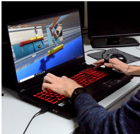
Figure 12: Operator's local computer with the open Mixed Reality GUI. The heartbeat and GSR sensors are worn on hands.
