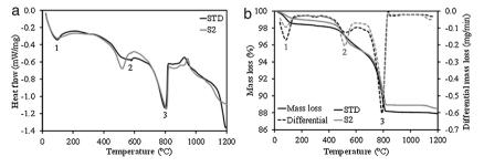
Fig. 2 – Simultaneous thermal analysis of the compositions STD and S2 (intermediate composition of those studied): (a) DSC, (b) TG.
