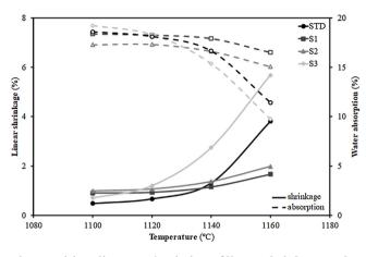
Fig. 3 – Firing diagrams (variation of linear shrinkage and water absorption of the pressed pieces with the maximum firing temperature) for the studied compositions.
