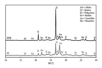
Fig. 6 – X-ray diffractograms of specimens fired at 1120°C of the compositions STD and S2.
