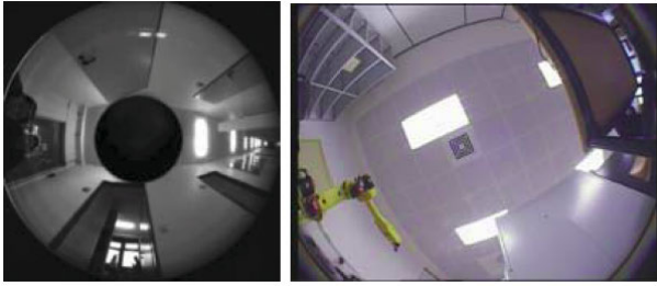
FIGURE 1. Difference between a catadioptric image (left) and a fisheye image (right).
