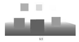
Fig. 3: Experimental setup. a) Relative position between Baxter robot and scenario. b) Layout of markers in the test scenario. c) Depth image generated by the simulator, using a virtual depth camera with the same intrinsic parameters than the RGB camera, and placed in the same position.
