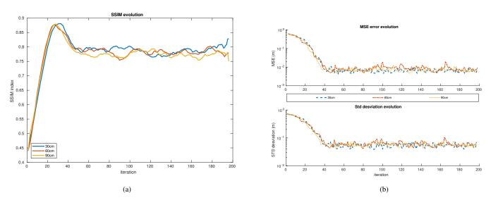
Fig. 11: Evolution of the algorithm results for fixation points at 30, 60 and 90 cm. a) SSIM evolution. b) MSE and STD evolution
