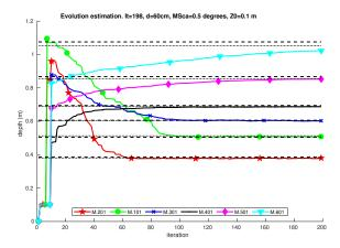
Fig. 9: Example of the evolution of depth estimate mean for the Aruco regions only, wit a fixation point at 60 cm. The dotted lines are the distances of the markers given by the simulator, and the dashed lines are the distances estimated by the Aruco algorithm.
