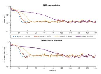
Fig. 4: MSE and STD deviation between the background depth image and the estimation made by the proposed algorithm for 60 cm fixation point and different values of  $\rho$  for a constant value of  $\sigma=0.01$
