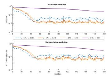
Fig. 5: MSE and STD deviation between the background depth image and the estimation made by the proposed algorithm for 60 cm fixation point and different values of  $\sigma$  for a constant value of  $\rho=0.70$
