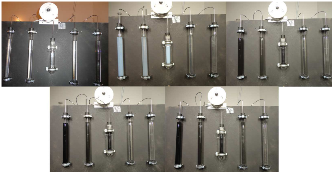
Figure 2 From left to right, from top to bottom: water, silica nanofluid, Chinese ink, carbon nanohorns + SDS and carbon nanohorns + SDS + PVP
