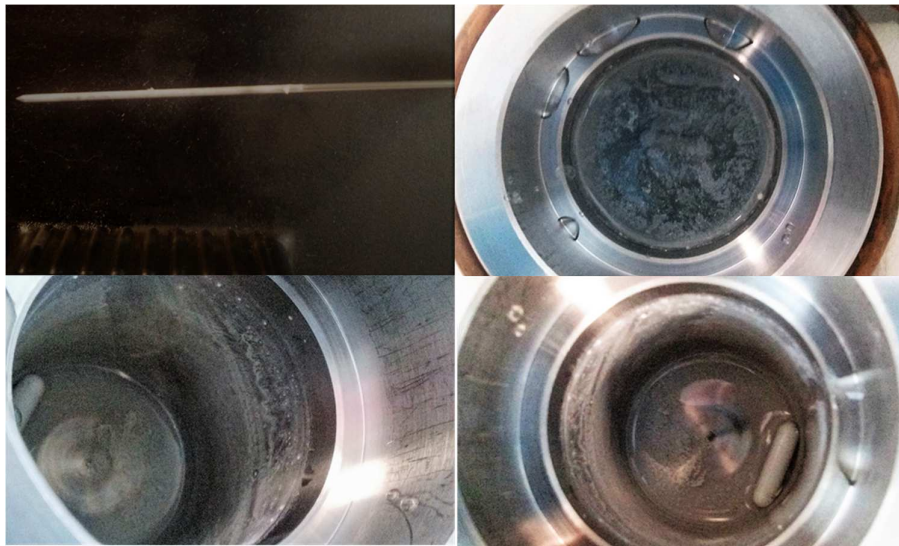
Figure 4. Visual inspection after thermal conductivity measurements with magnetic stirring (top left image showing the probe and all others showing the container).
