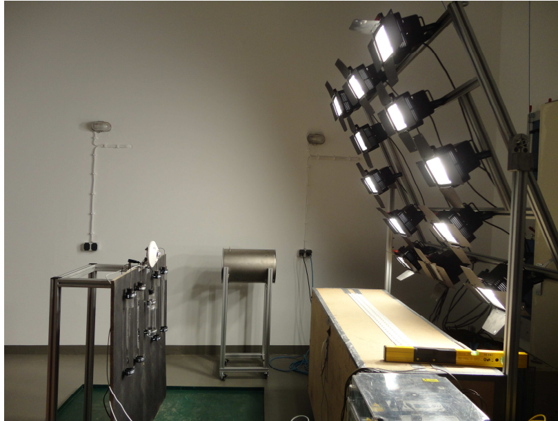
Figure 1 Lamps structure imitating an artificial sun lighting the samples
