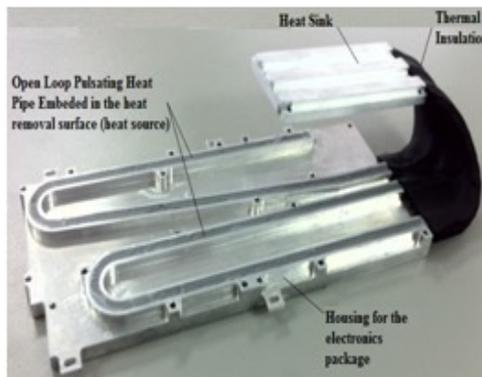
PHP schematics for electronics cooling.
