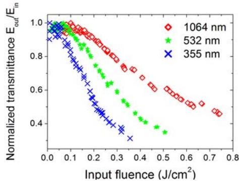
Normalized transmittance, i.e. the ratio between output and input energies, normalized to its maximum value of nanodiamond suspensions with 0.005% wt concentration at 355, 532 and 1064 nm light wavelength [1]. In the linear regime, the normalized transmittance is unity, and decreases in the optical limiting regime.
