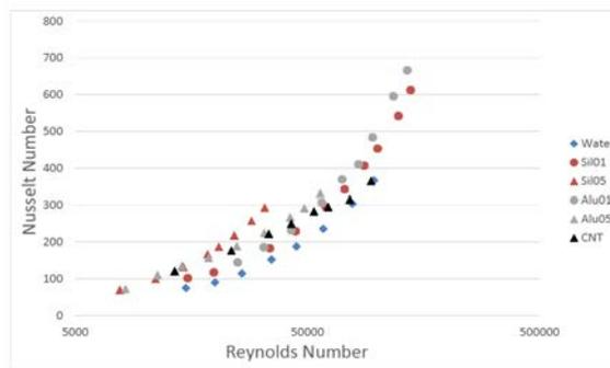
Heat transfer performance of water based nanofluids with silica (1 and 5% w.t.), alumina (1 and 5% wt) and carbon nanotubes (0.125% wt). At a same nanoparticle concentration, CNTs provide the highest differences because of their huge viscosity increase. Alumina provides the lowest differences as they show the smallest viscosity increase.
