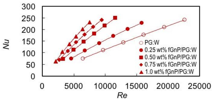
$Nu$  versus  $Re$  for functionalized graphene nanoplatelet (fGnP) dispersions in propylene glycol:water 30:70 wt% mixture (PG:W) [2]
