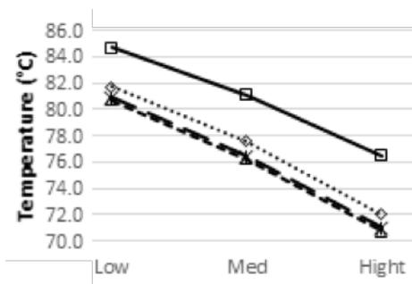
Outlet radiator temperature for different nanoparticles concentrations.
