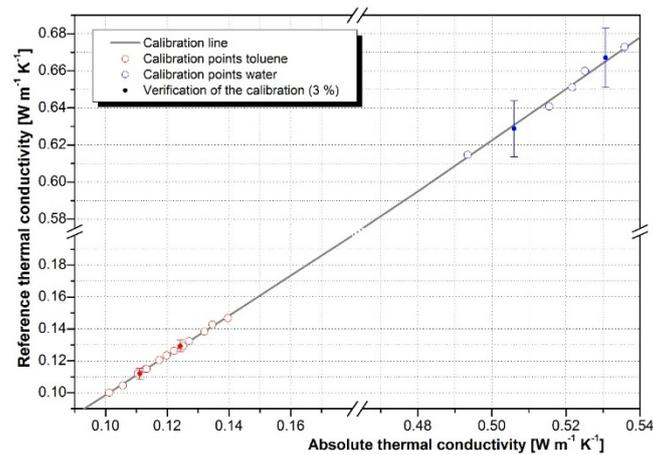
Calibration / verification of the measurement device
