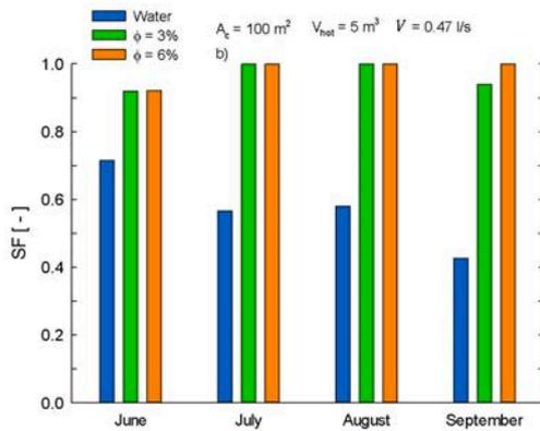
Solar fraction values at different months for several nanoparticle volume concentrations and solar field area values.
