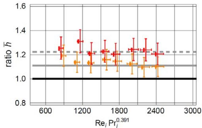
Ratio of heat transfer coefficients (nanofluid / water).
