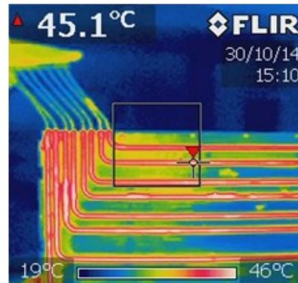
PHP infrared operation showing heat transport (temperature).
