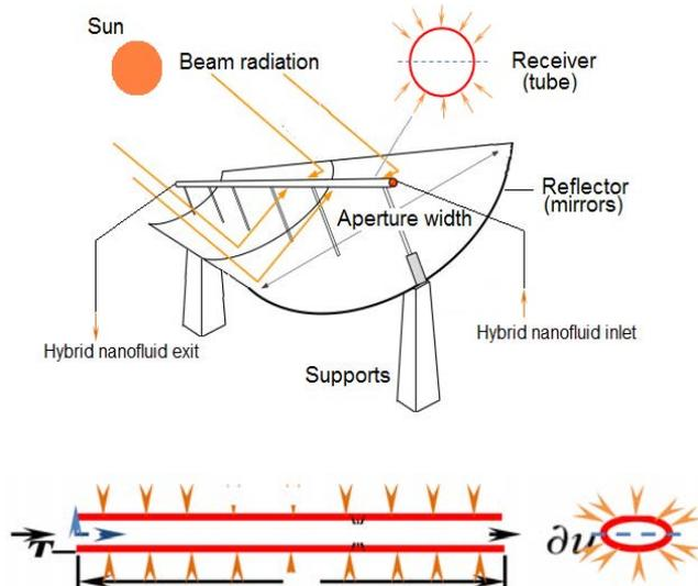
A view and a schematic diagram of the problem showing coordinates orientation with the hybrid nanofluid flow inside the tube of the parabolic trough.
