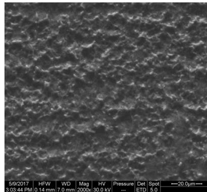
Figure 2: Coated (BOTTOM) surface after Cu/water nanofluid boiling on the copper surface.
