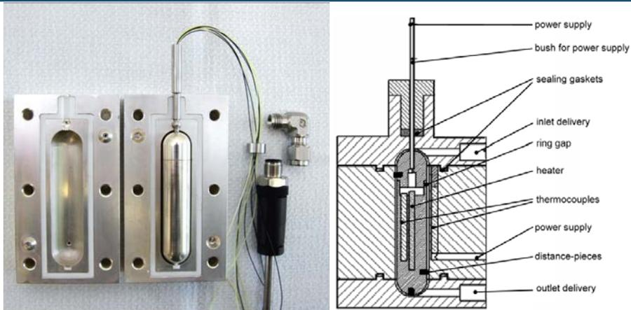
Ring gap apparatus made of silver (left) and main parts of device [1]
