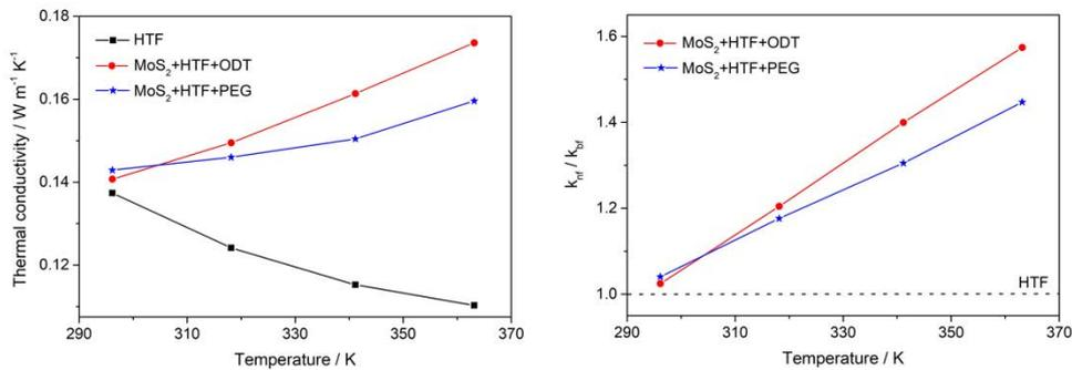
Thermal conductivity and thermal conductivity enhancement for nanofluids based on 2D-MoS<sub>2</sub> using ODT and PEG as surfactants.
