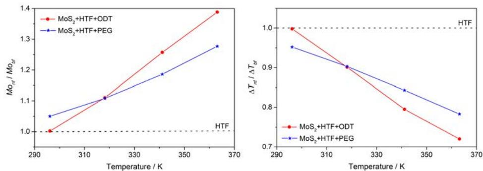
Mouromtseff number ratio of the nanofluids based on MoS<sub>2</sub> and the base fluid; and the analysis of the outlet temperature in solar collectors.
