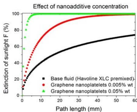
Extinction of sunlight  $F(x)$  as a function of the path length  $x$  within the nanofluid.  $I(\lambda)$ : sunlight spectrum;  $\alpha(\lambda)$ : nanofluid spectral extinction coefficient;  $\lambda$ : wavelength;  $\lambda_{\min}=300$  nm;  $\lambda_{\max}=3000$  nm
