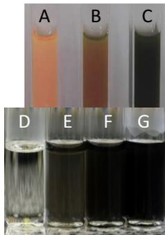
(A) pure base fluid (Havoline XLC premixed); (B) Base fluid with 0.005% wt graphene nanoplatelets; (C) Base fluid with 0.05% wt graphene nanoplatelets (samples provided by L. Lugo, University of Vigo, Spain); (D) pure base fluid (ethylene glycol); (E) Base fluid with 0.0025% wt graphite/nanodiamond mixture; (F) Base fluid with 0.0050% wt graphite/nanodiamond mixture; (G) Base fluid with 0.0100% wt graphite/nanodiamond mixture (samples provided by G. Zyla, University of Rzeszow, Poland).
