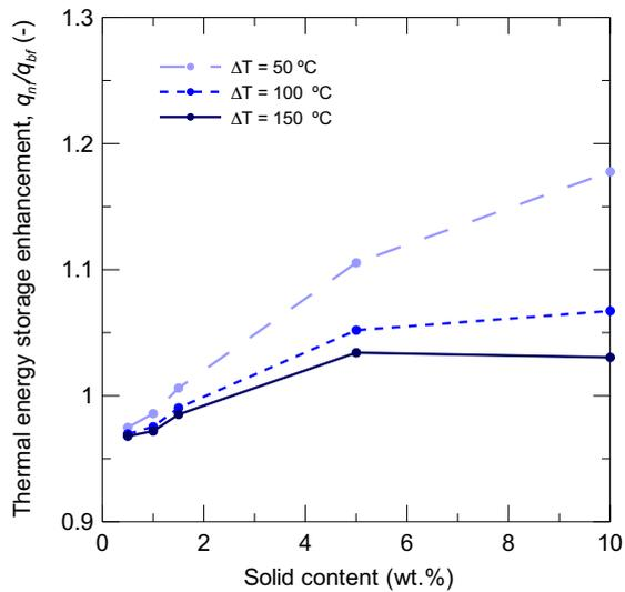
Evolution of the total thermal storage enhancement with solid content of Al-Cu nePCM on a constant volume basis.
