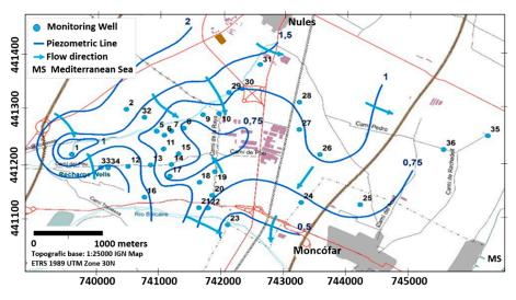
Figure 2. Piezometric map of the Rambleta area, October 2012 (modified from [40]).
