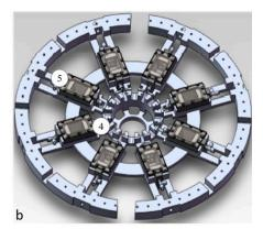
**Figure 1.** Prototype core details in cross-section (**a**) and 3-D view of MCW (**b**): (1) permanent magnet assembly; (2) magnets support; (3) shaft-rotary valve combination; (4) regenerators; (5) magneto caloric wheel (MCW); (6) cold sub-valve and (7) hot sub-valve.
