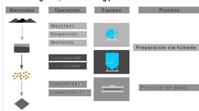
Figure 5; Manufacturing process of ceramic tiles
