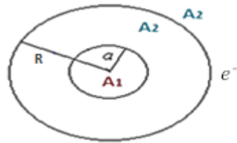
Figure 3: Scheme of the one-dimensional ring of radius R and with inner radius a and inner circle pierced by an axial magnetic field.
