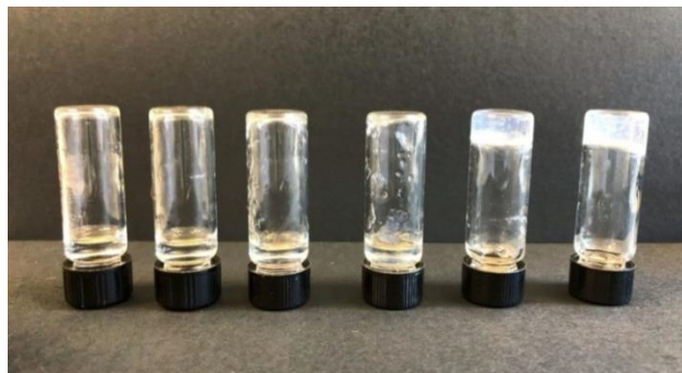
Figure 3-7. Vial inversion test for Ratio DMSO:H 2 O 10:90 . Left to right concentrations (mM): 0.5 - 0.6 - 1.1 - 1.5 - 1.6 - 2. It is shown that the gel is formed above 1.6 mM. Images for the ratio DMSO:H 2 O 5:95 are not included, but the same criterion was followed.
