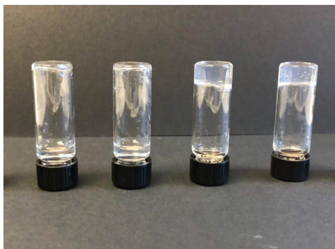
Figure 3-10. Vial inversion test for ratio DMSO:H 2 O 10:90 at pH 9. Left to right concentrations (mM): 0.7 - 0.8 - 1 - 1.5.
