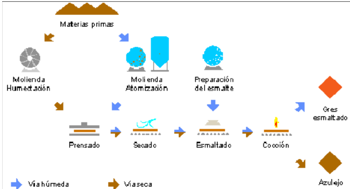
Picture 8 Manufacturing process of ceramic tiles
