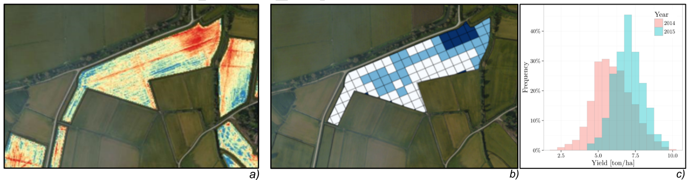
Fig. 9. Examples of a) ERMES field variability products (red colours correspond to lower crop vigour), b) prescription maps derived from their analysis (darker blue corresponds to higher nitrogen amount to be provided), and c) comparison between frequency distribution of final yield in the field between 2014 and 2015.
