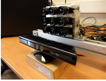
Fig. 2. The two sensors used in the experiments: the 3 \times 3 camera array on top and the Kinect below
