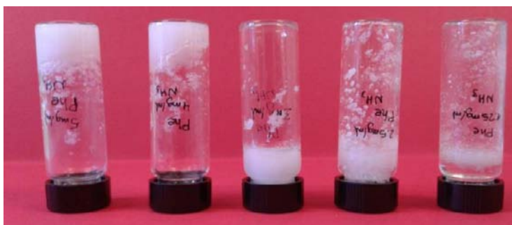
Figure 3-5. SucPheDoc inversion tube test from highest concentration (left) to lowest concentration (right).
