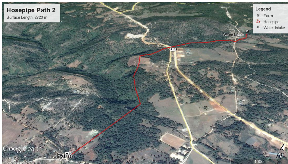
Figure 20. Hosepipe path 2 (surface length 2,723 m)
