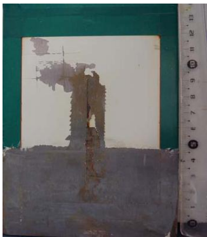
Fig. 3. Photograph of the Reference panel after 641 hours in the salt spray chamber.
