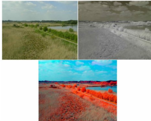
Figure 20. Digital images in natural color (top left), near infrared (top right) and the color infrared composite (bottom) (Knoth et al 2011).
