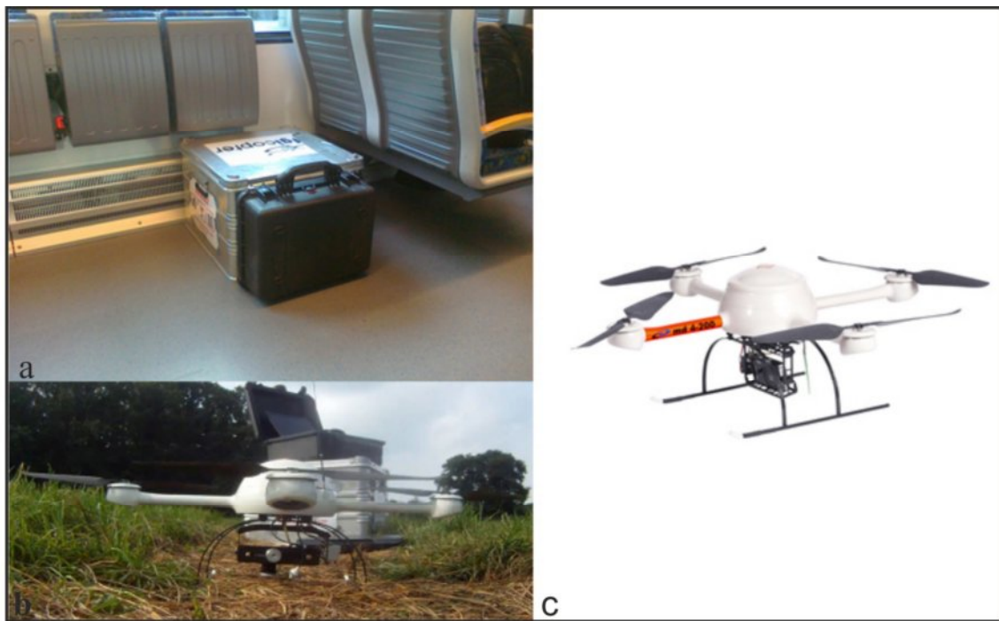
Figure 12. a) quadcopter microdrone md 4-200 and ground station in transportation boxes, b) quadcopter microdrone md 4-200 and ground station with modified digital camera (Canon PowerShot SD 780 IS), c)quadcopter microdrone md 4-200 (Microdrone 2014).
