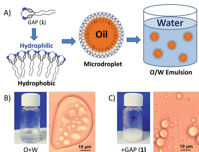
Fig. 2 (A) Schematic representation of the self-assembly of the GAP ( 1 ) toward the formation of an o/w emulsion. (B and C) Macroscopic and microscopic pictures of the oil–water mixtures (O + W) alone (B) and after the addition of the GAP and 30–90 minutes of vigorous stirring (C).
