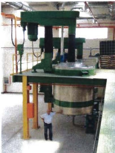
Dissolver *MASTERMix*\* 160 with stationary 10 000 liter tank for mezzanine assembly
