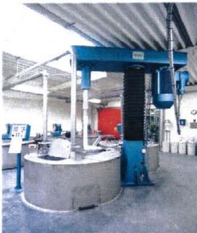
Swivel-type Dissolver *MASTERMix*\* 110 for mezzanine assembly
