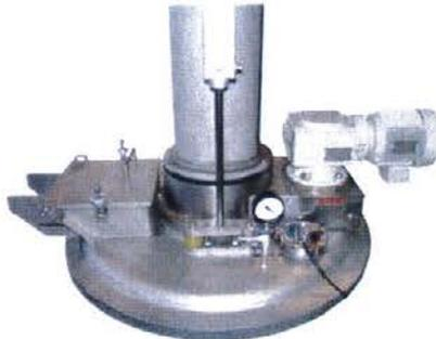
Vacuum tank cover with scraper drive
