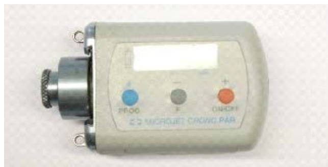
Figure 1: The subcutaneous pump is used for dynamic drug delivery. The pump has been modified to receive commands via a ZigBee interface
