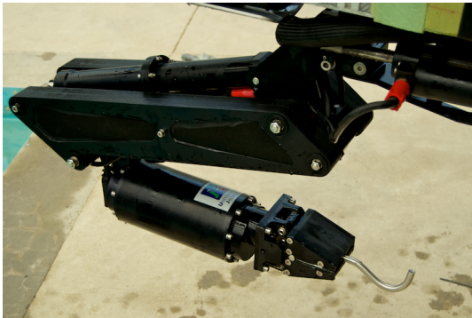
Fig. 3 The Light-Weight ARM 5 E with a hook attached to the gripper. The T-shape grooves of the gripper allow attachment of different tools depending on the application.
