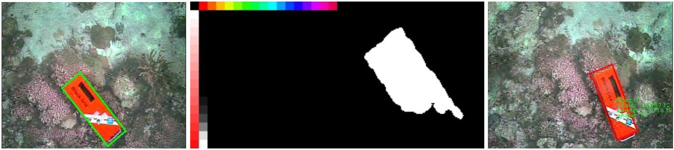
Fig. 9 Left : image from the survey stage on which the model of the target is based. Center : model of the target based on the bidimensional HS histogram. Right : detection, pose and size estimation of the target.
