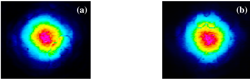
Figure 10. Experimental irradiance distributions at the sensor plane when the codified focal length at the SLM are 22.5 cm (a) and 23 cm (b).
