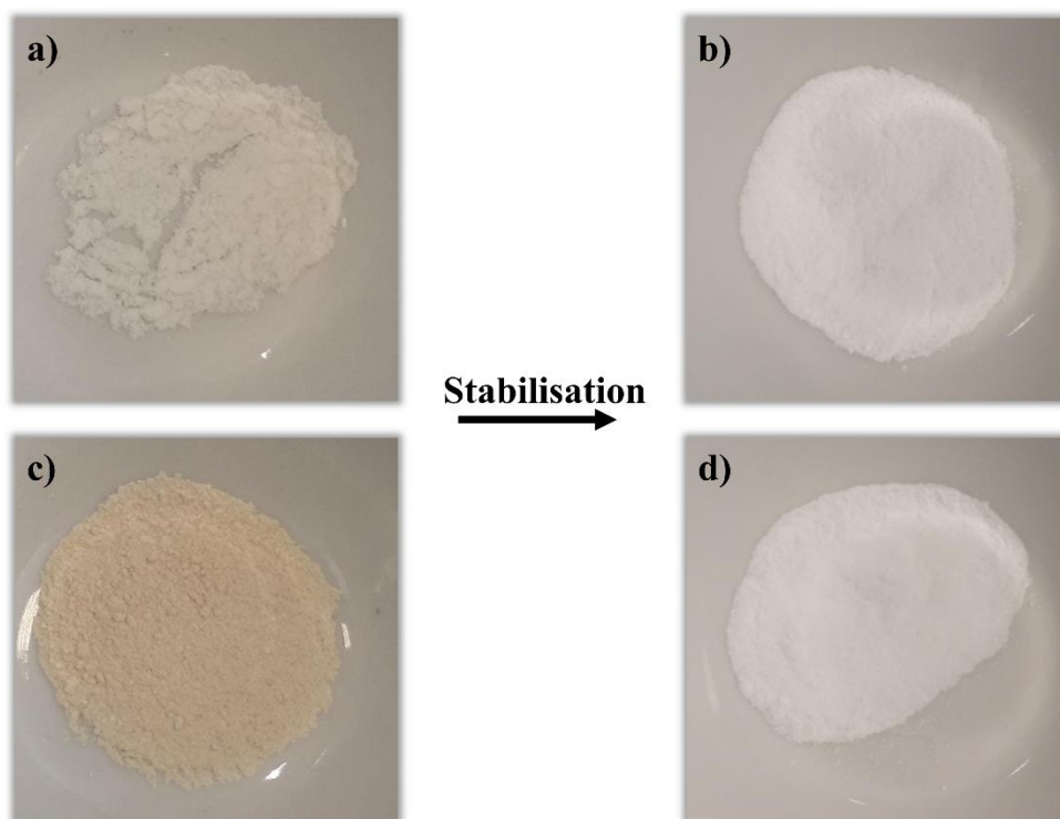
Figure 2. Images of the xerogel powders before and after thermal stabilisation. a) and b) G1 (170°C-18bar-40min) before and after stabilization, respectively, c) and d) G2 (190°C-35 bar-40 min) before and after stabilization, respectively
