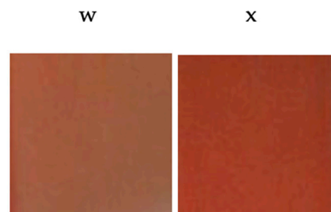
Figure 17. Color development of glazed tiles with pigment Y_{0.98}Al_{0.98}Cr_{0.04}O_3 with flux agent mixture fired at (w) 1400 °C/2 h; (x) 1400 °C/6 h.
