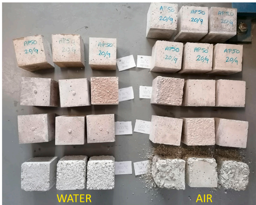
Fig. 9. Photographs of the CSFA50 specimens after being exposed to different temperatures and cooled in water and in air.
