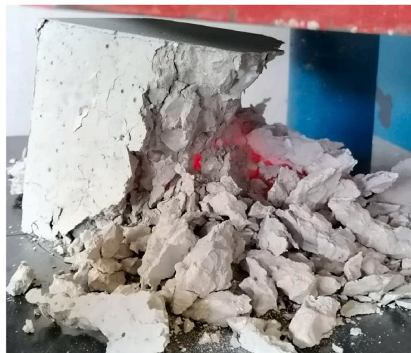
Fig. 8. Broken sample after hot testing at elevated temperature.
