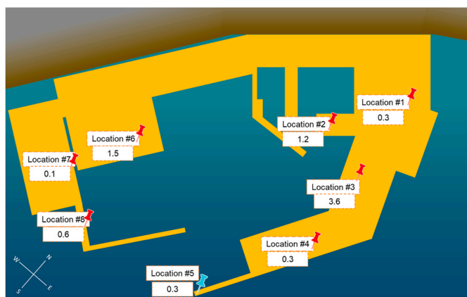
Fig. 8. Map of PM 10 concentrations (measured by laser spectrometry) at the different locations, reported as the ratio between monitored concentrations and average concentrations across locations and over the full period.
