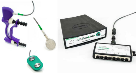
Fig. 3. Hand grip and pinch dynamometers, sEMG electrode (SX230) and 8-channel sEMG Biometrics Ltd. devices.
