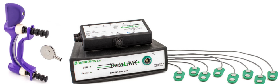
Figure 2. Hand grip and pinch dynamometers, sEMG electrode (SX230) (Biometrics Ltd., Newport, UK) and eight-channel sEMG Biometrics Ltd. devices, (Newport, UK).
