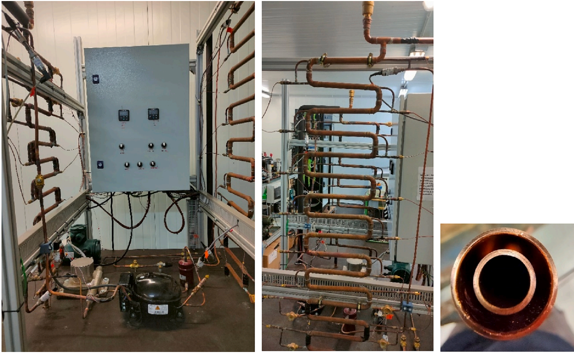
Fig. 2. Different pictures of the test bench before the application of heat insulation. From left to right: a general picture of the machine, followed by a focused view of the condenser, and finally, the cross section of the evaporator.
