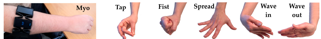
Figure 2. Myo armband and recognized hand postures from proprietary software Myo Connect version 1.0.1.
