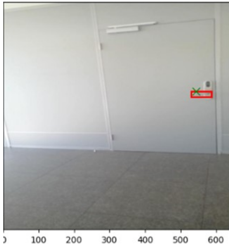
Figure 5.8: Grip point for door handle that opens to left size generated for the euclidean geometric model, with coordinates in same framework.
