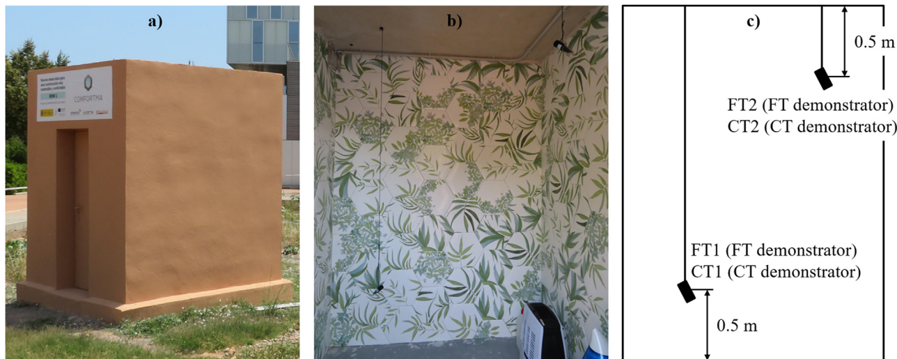
Fig. 2 – Images of the demonstrator FT: (a) exterior, (b) interior and (c) mounting diagram for humidity sensors.
