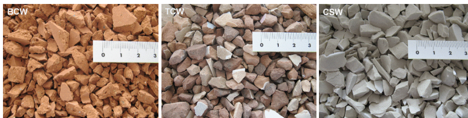
Figure 2. Crushed CW particles obtained from bricks, tiles and sanitary ware.
