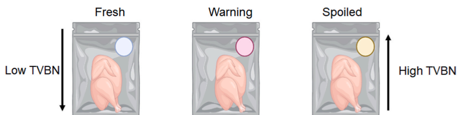
Fig. 3. Application of smart film in chicken quality monitoring. TVBN: Total Volatile Basic Nitrogen.
