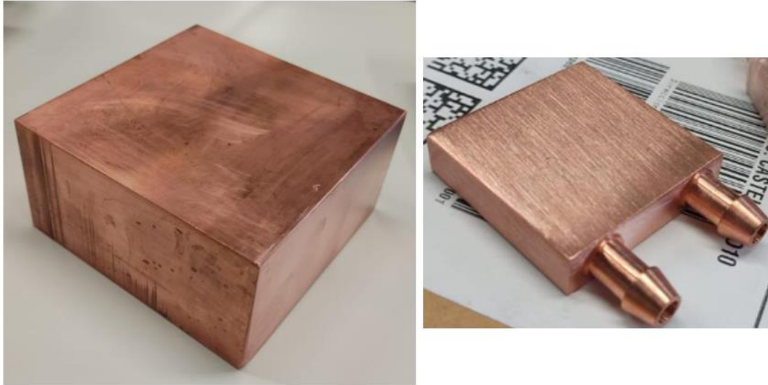
Figure 18. A) Solid copper block. B) Smaller block with water circulation.
