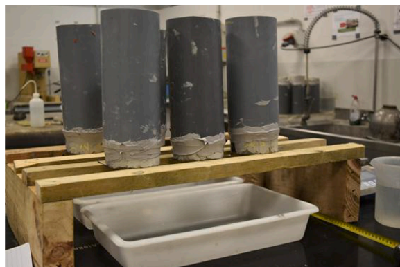
Fig. 2. Water permeability test setup, diagram, and photo of the setup.
