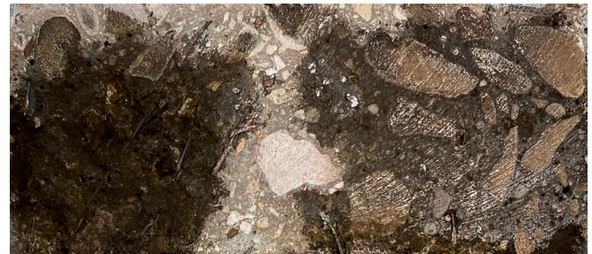
Fig. 8. Effect of ITZ on chloride penetration of conventional concrete specimen.
