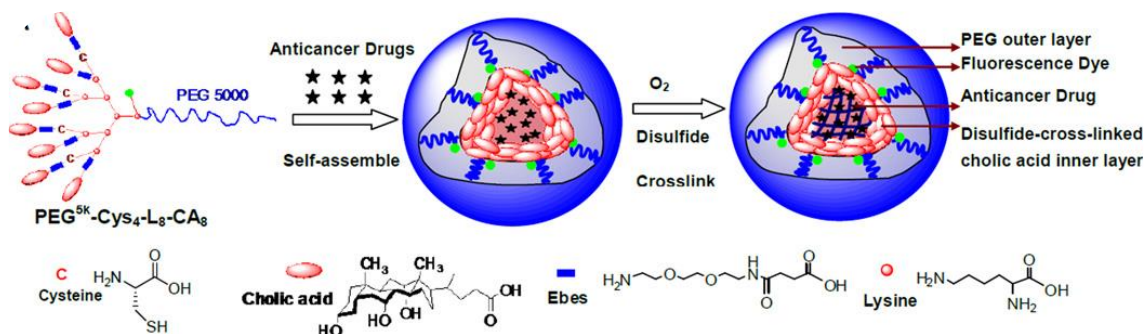
Figure 1.13: Schematic representation of disulfide-crosslinked micelles formed by the oxidation of the thiolated telodendrimer \text{PEG}5k\text{-Cys}4\text{-L}8\text{-CA}8 after self-assembly. 15
