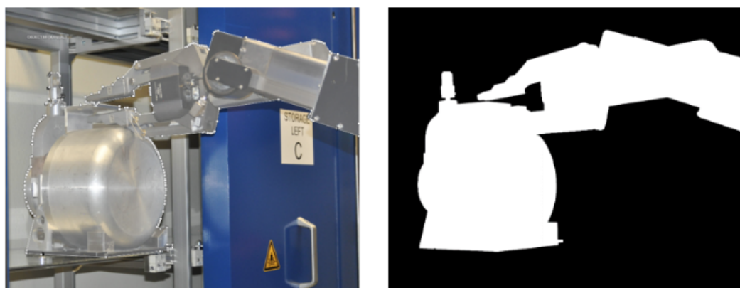
Figure 5. Labeling process: (left) segmentation by the hand of the interest object. (right) Mask after segmentation.
