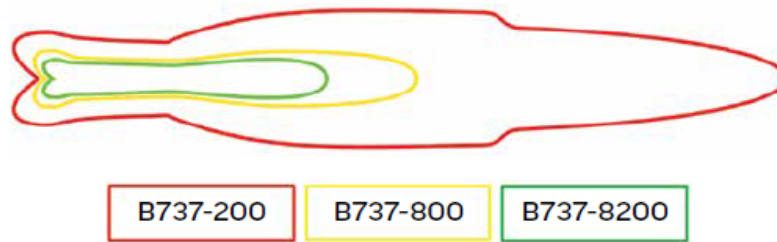
Figure 11: The new Boeing 737-8200's noise compared to previous fleets
