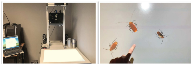
Figure 2 Images depicting the projection-based augmented reality exposure treatment system and an example of how the cockroaches look like from the patient's view.
