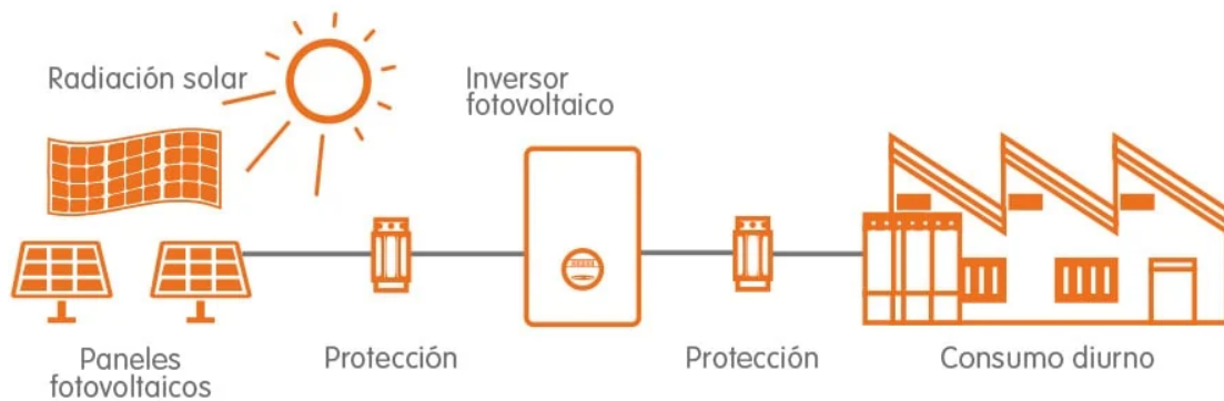
Figure 10. Elements of a solar panel installation.
