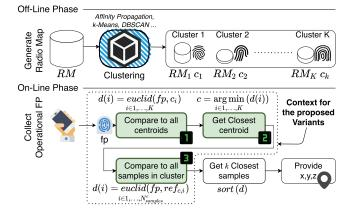
Fig. 1. Fingerprinting with clustering.
