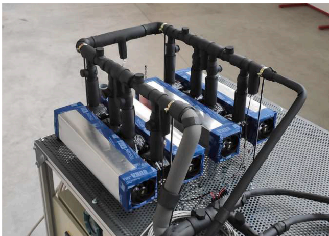
Fig. 6. Experimental thermoelectric subcooler.
