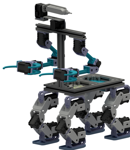
Figure 29. An alternative design with four legs like a centaur that a student designed for an environment with rocks.
