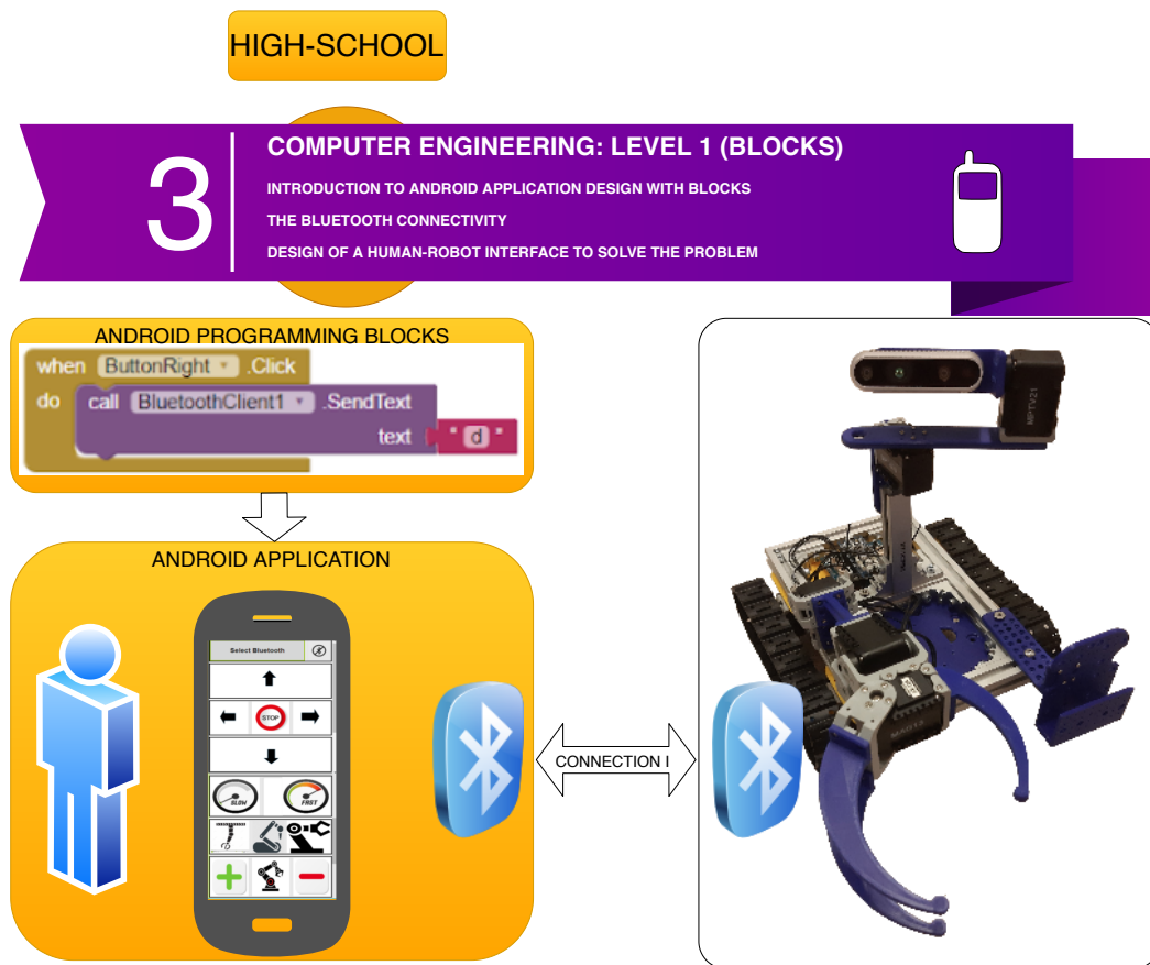
Figure 13. Software architecture for the Computer Engineering Level 1 exercise.
