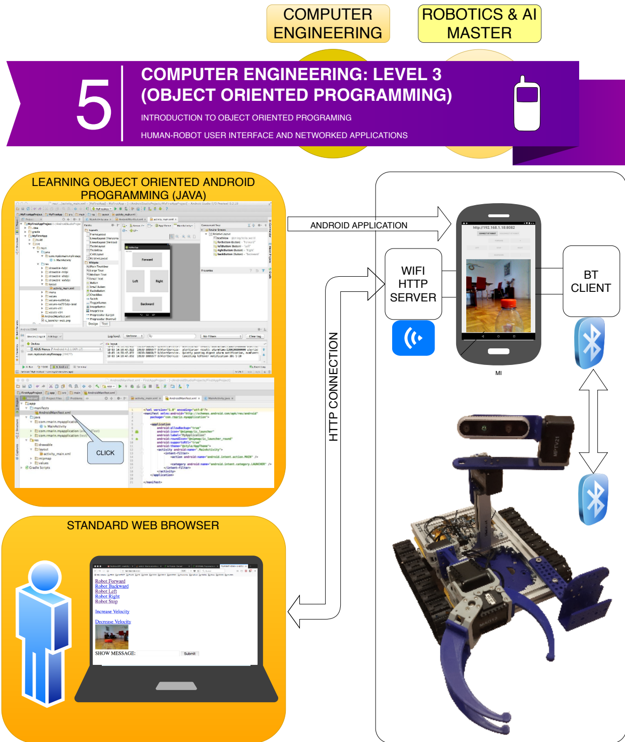
Figure 18. Software architecture to face the Level 3 learning path (i.e., Object-oriented Programming).
