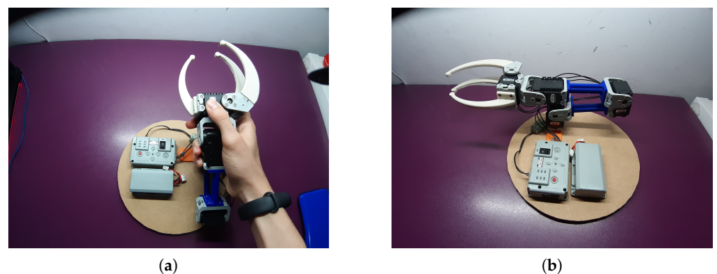
Figure 27. Student Project to implement a Master-Slave system to control the robot arm at a distance. (a) Frontal view, (b) side view.
