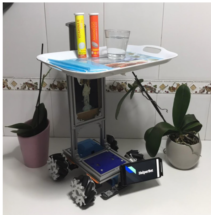
Figure 31. Helper Bot, MiniCernBot's configuration for medicine applications.
