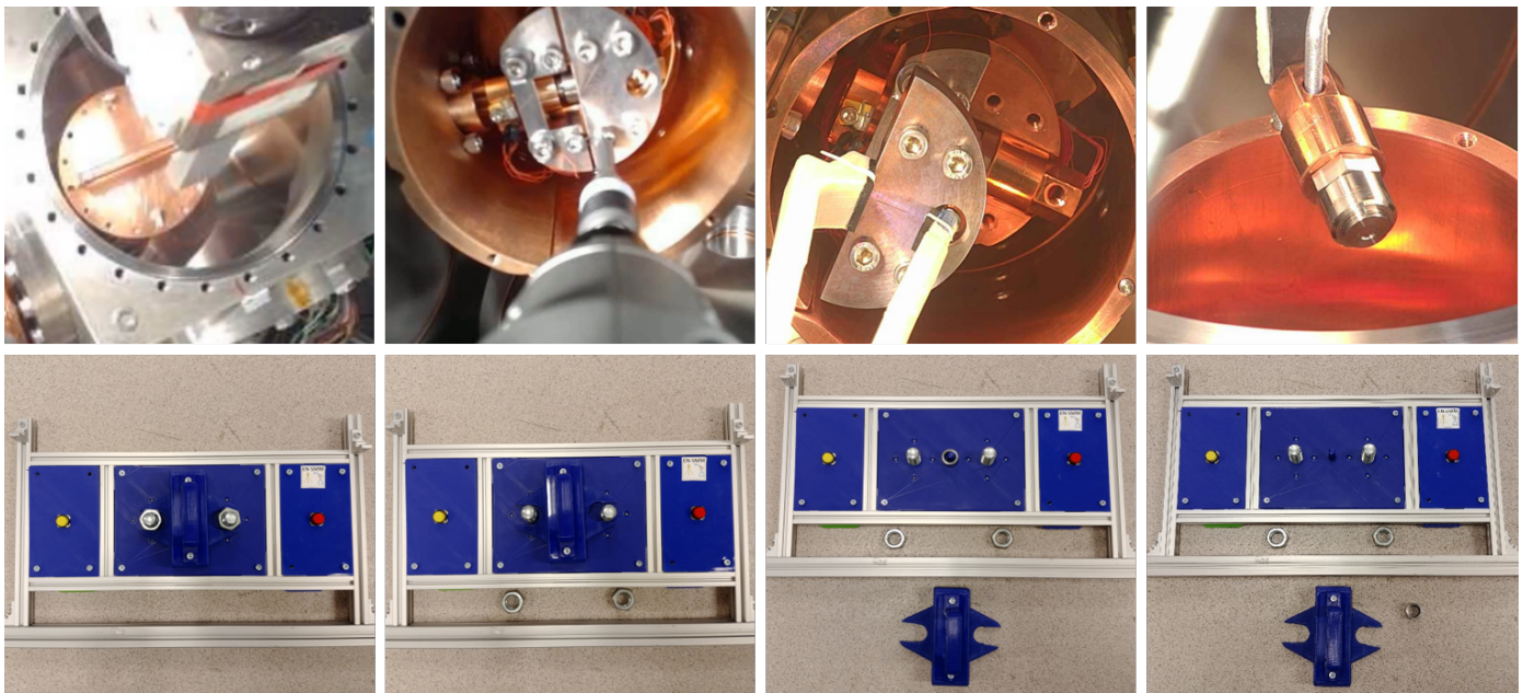
Figure 2. (First row) Antimatter factory real intervention performed by the CERN-EN-SMM-MRO team to recover a radioactive source; (Second row) Educational Mockup simulating the necessary steps to recover a source.
