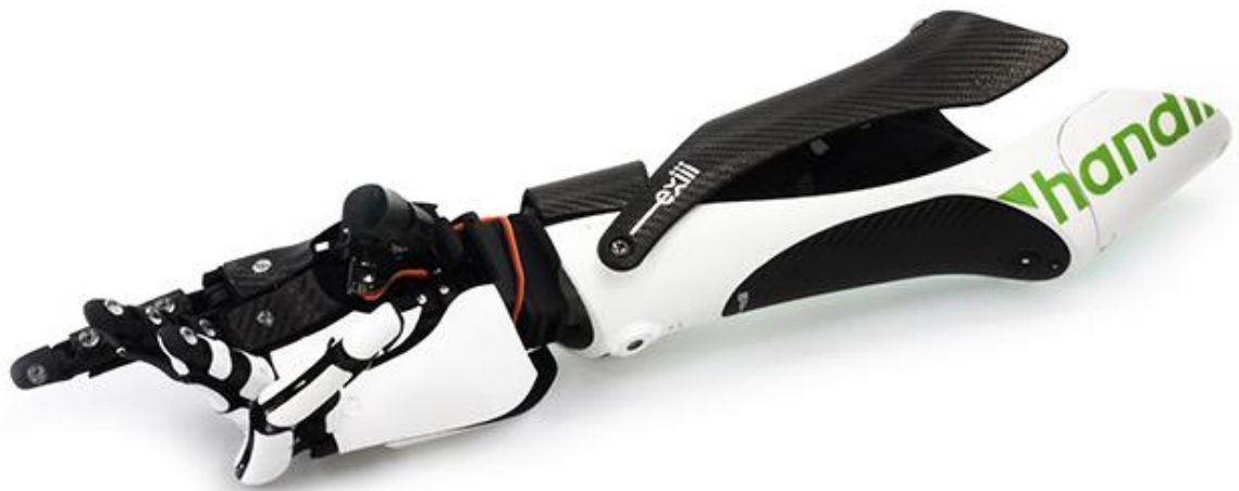
Figure 10 handiii COYOTE myoelectric prosthesis [17]
