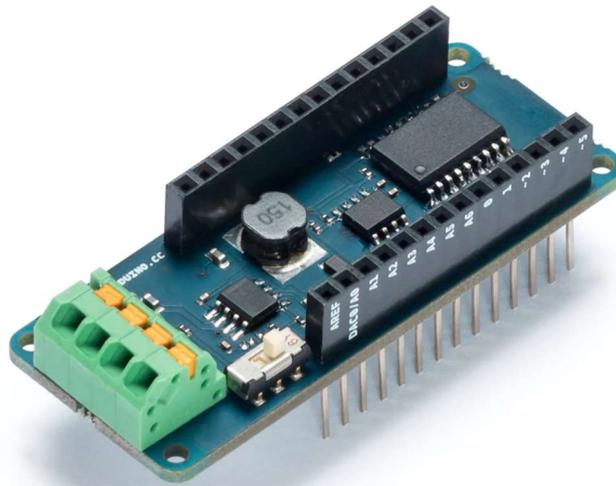
Figura 46. Placa Arduino MKR CAN Shield [14]
