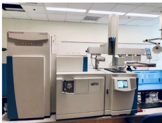
Figure 4. Gas chromatograph coupled to HRMS with autosampler used in the project
